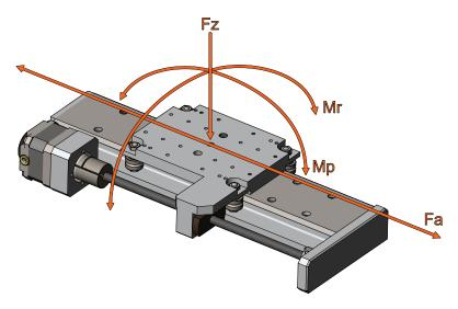
**MATERIALS:** The major components of standard stages are manufactured from 6061 T6 aluminium. The material surface is processed to obtain a thin, dense aluminium oxide coating which reduces diffusion and desorption at UHV. A 304L stainless steel version can be specified using option code "SS".
