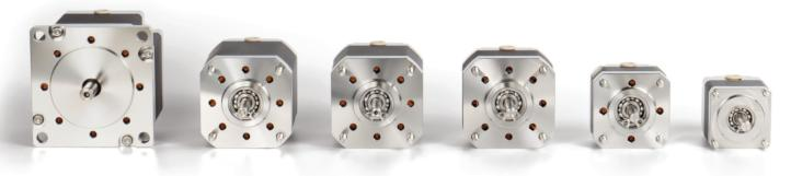
The model D motors are two phase hybrid stepper motors, available in a range of standard sizes and torque ratings. Standard motors provide 200 full steps per revolution, are suitable for use below  $1\times10^{-10}$  mbar and working temperatures between -65 °C to +190 °C. Extended low temperature range (-196 °C) versions, radiation hard versions (1 x  $10^6$  Gy), shaft modifications and hybrid bearings are all available options.
